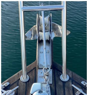
The installed setup on Nirvana, I think thread-lock is more reliable than locking wire (but invisible) so I used both when I finally obtained some bright annealed Tp316 stainless steel locking wire. The swivel part is welded, not just screwed as the hexagons make it look!
